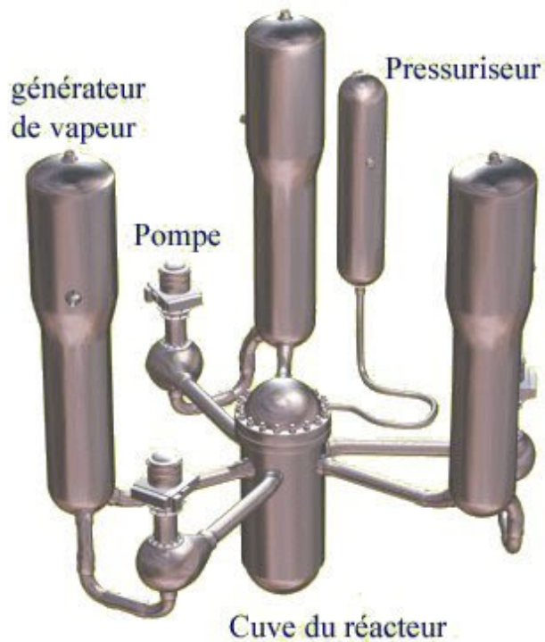
Figure 9: Illustration du circuit primaire
